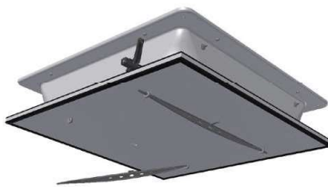
Step 5: (Install Lid to Inlet)
