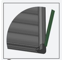
Install the cover clips onto profiles (sides and top only)
