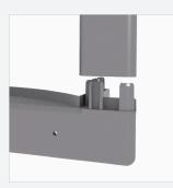
**Step 2.** Install long frame section with hinge profile onto side endcap.
