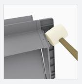
**Step 6.** Using a rubber mallet, be sure endcaps are securely in place.
