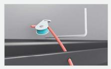
**Step 7**. Pull string through hole in louver, then through block or pulley towards direction of pull.
