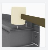
**Step 7.** Using a rubber mallet, install eight plastic nails in holes, securing inlet together.
