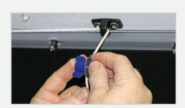
With actuator in closed position, adjust so lids are closed.
