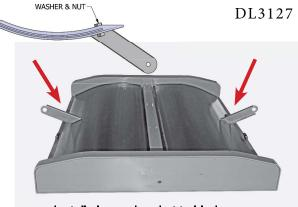
Install closure bracket to blade using hardware supplied.
