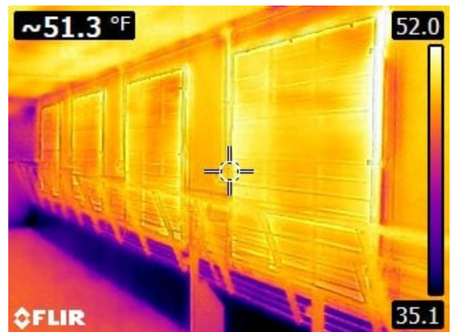
Above FLIR photo was taken at the same finishing site in eastern Iowa 15 minutes after the Shutter Blank was installed on the 54" fans.
