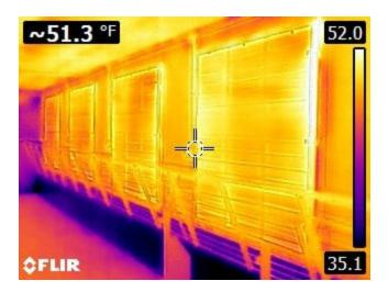
Above FLIR photo was taken at the same finishing site in eastern lowa 15 minutes after the Shutter Blank was installed on the 54" fans
