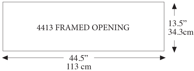
Step 1 Install inlet into the framed opening.
